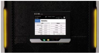
Yellow light bars indicate battery or bypass.
